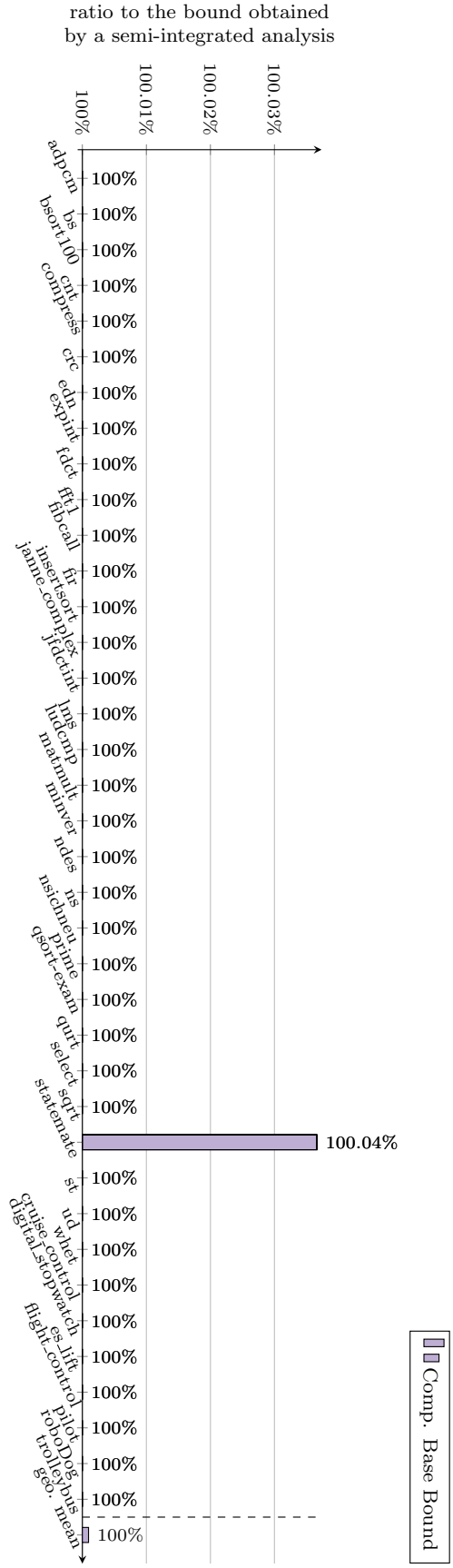
Figure 48: Ratio of the compositional base bound approach to the semi-integrated timing bound with no interference. The results of the other approaches agree with the semi-integrated bound under the absence of interference. Configuration 1, quad-core processor.
