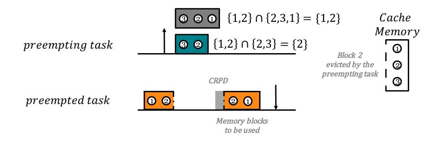
Different preempting tasks cause different CRPDs due to eviction! 5
