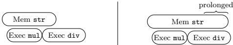
Figure 5: The execution of two subsequent arithmetic instructions hiding the latency of a preceding store.
