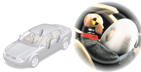
Side airbag in car Reaction in < 10 msec
